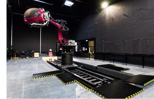
The large motion range of the CyberMotion Simulator allows pilots to experience unusual attitudes in motion. Foto: Victor S. Brigola
